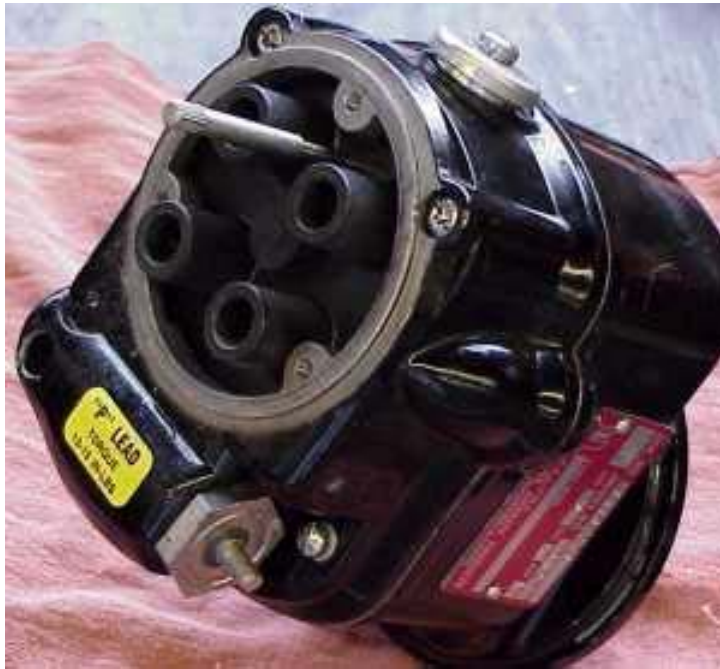
Slick magneto showing the timing pin inserted.
