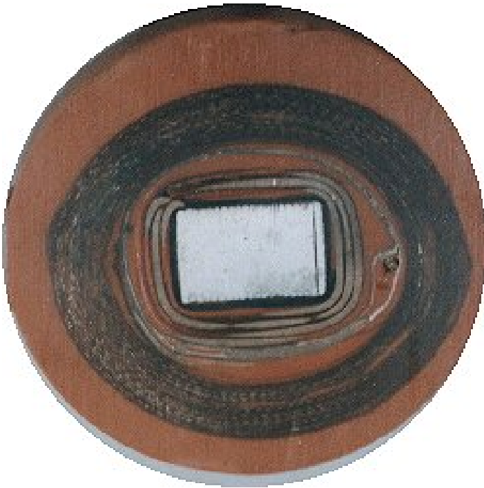
Slick coil x-section showing the primary coil (thicker wire) and secondary coil (thinner wire) wrapped around the laminated iron core.
