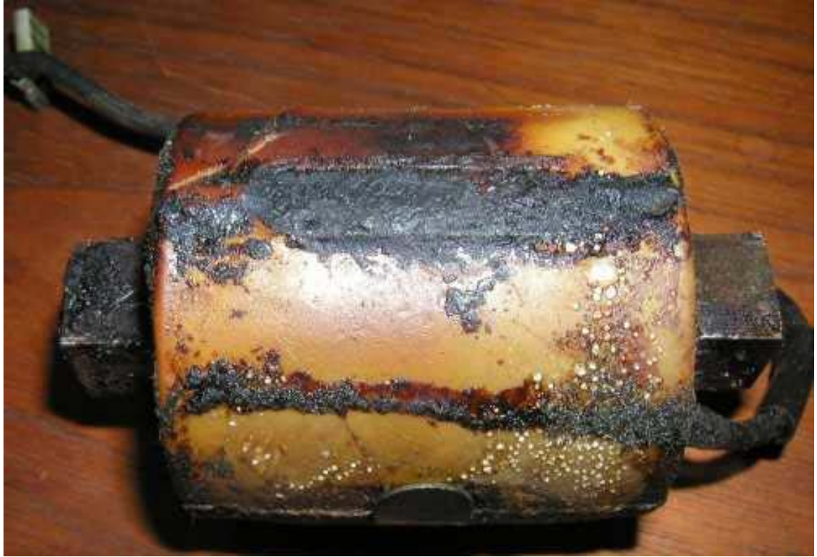
Badly neglected Bendix coil
