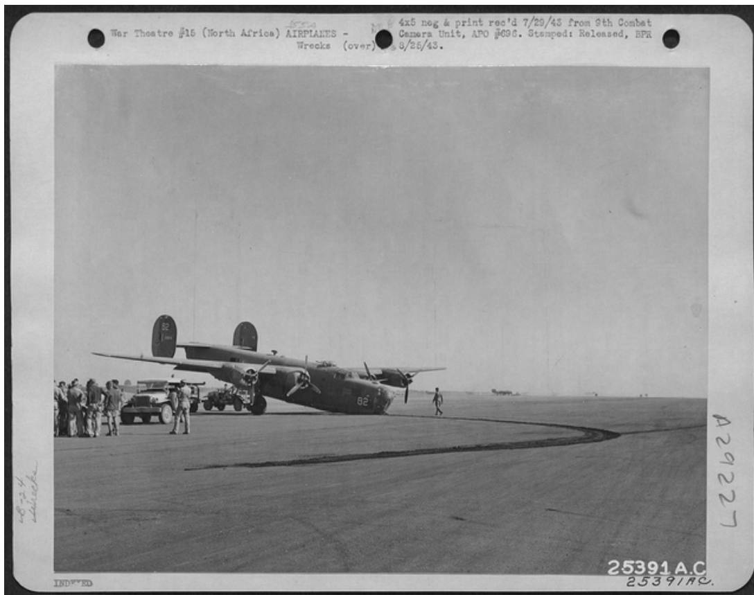
Figure 1. A B-24 Liberator, shown after suffering a nose wheel failure at a base in North Africa. Nose wheel shimmy was a serious enough problem that all the Halpro aircraft carried a spare nose wheel when they left Florida.
