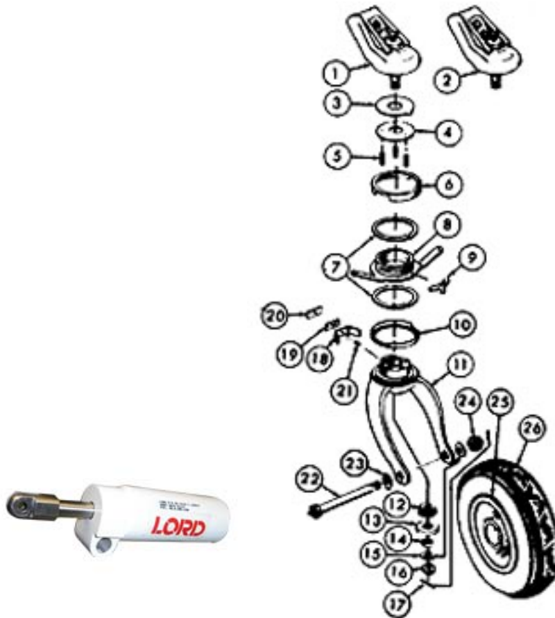
Figure 3 shows examples of shimmy dampeners. The Lord shimmy dampener is most commonly used on aircraft nose wheels. The integral spring loaded pressure plate dampener is common on Scott tailwheels.
