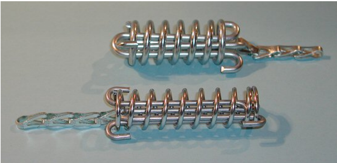
Figure 4 Rudder springs of two different sizes used to supposedly help dampen tail wheel shimmy. The larger stiffer spring is typically used on the right rudder to help counter left turning tendencies.
